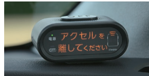
Display of the retrofit Pedal Misapplication Acceleration Control System II
