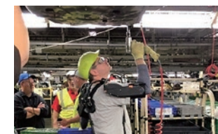
Example of improvement: A power assist device to reduce arm fatigue (North America)
